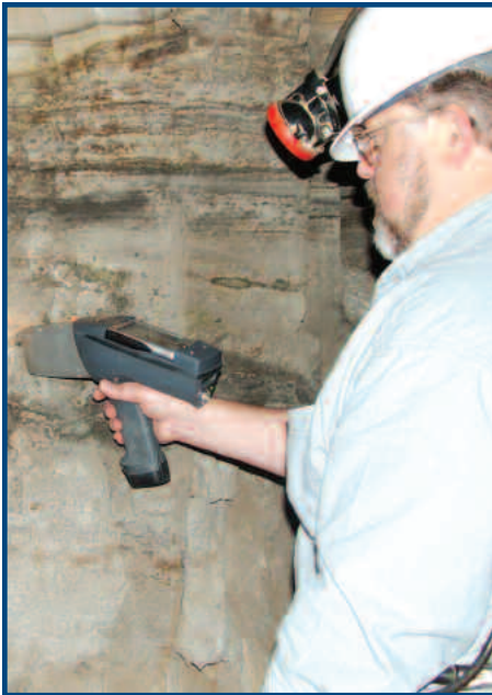
Alpha Series™ achieves fast, on-the-spot results for elemental analysis of P-U for mine mapping and on-site geochemical exploration.
