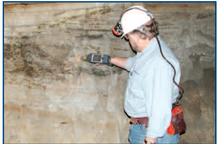
In-situ survey of mine tunnel used for ore mapping. Alpha Series™ can also evaluate uniformly homogenized samples for comparative lab analysis.
