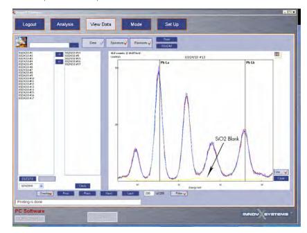
A reference sample spiked with approximately 500ppm Pb (Innov-X sample 408) was used for these repeat readings.
