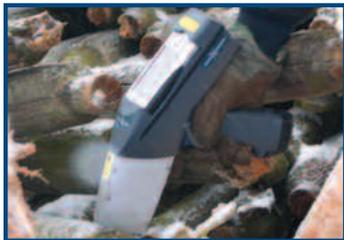
Alpha Series™ XRF analyzer enables fast site survey for on-site analysis of As and Pb.
