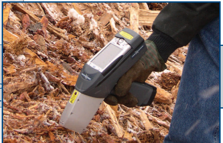
The Alpha Series™ identifies toxic metals, RCRA and other pollutants in a variety of samples.
