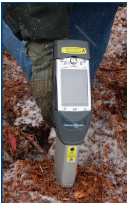
On-site analysis for CCA-treated wood is used to prevent recycling it into mulch.
